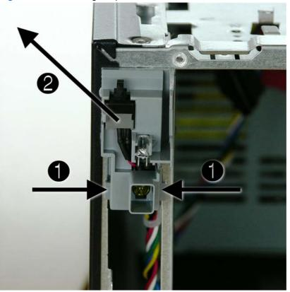
Figure 2-44 Removing the power switch
